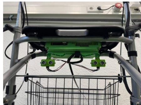
Figure 19: Prototype Rollator Integration of Sensors and Processing Hardware.
